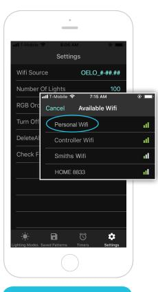
Please note that the controller only works on 2.4GHz WiFi network. The controller will not connect to a 5GHz WiFi network. **Step 2:** Enter your personal WiFi name and password exactly how it appears (may be located on your router).
